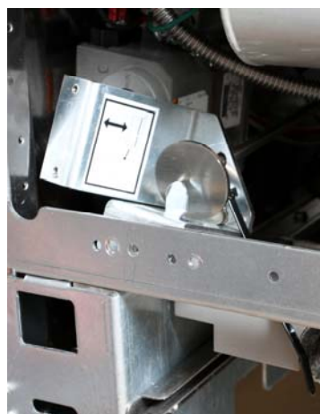
Figure 2: Loosen the disposal handle assembly and move to the side of the cabinet.
